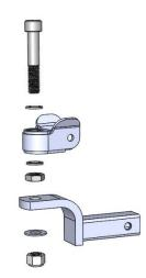
To set up your Max Coupler, you will need either our Adjustable Channel Mount (MC212) or a ball mount that puts the mounting surface at the height you need for your trailer.
