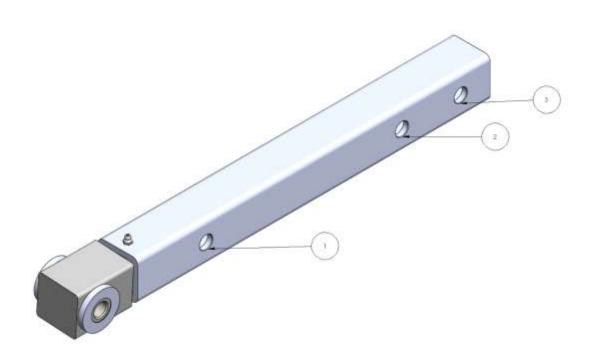
HOLE # 1 IS OUR ORIGINAL LENGTH MAX COUPLER. DO NOT ADD ANY HOLES TO THE LEFT OF THIS HOLE
