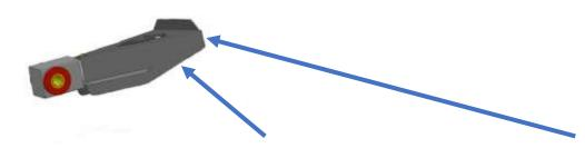
WELD ALONG THE ENTIRE BOTTOM ANGLED EDGE THAT MEETS THE FRAME, AND THE 1" STRAIGHT UP SECTION ON BOTH SIDES.
