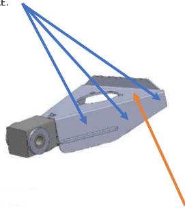
TO MEET THIS REQUIREMENT, THEY CAN ALSO BE DRILLED THROUGH THE TOP OF THE COUPLER IF YOUR TRAILER FRAME ALLOWS.
