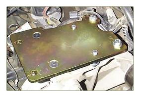
This adapter plate mounts our York compressor EF210R in place of the stock AC compressor on 4.0 and 2.5 engines. Our serpentine clutch 25-513352 and a longer serpentine belt (not included) will be needed to complete the installation of the compressor.
