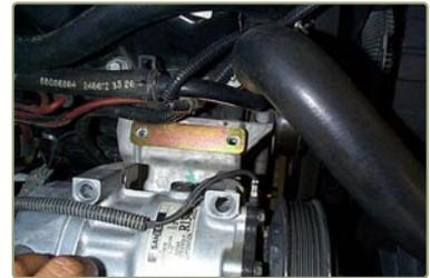
4. Reinstall the alternator and torque bolts to 41 ft lbs. Do not tighten the serpentine belt at this time.
